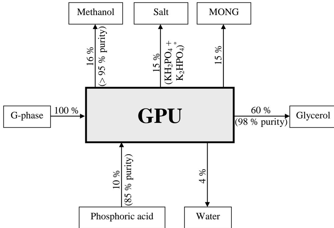
\* Salt is shown as pure. In reality it is dissolved in water for easy transportation and a potential to apply it directly as a liquid fertilizer.
